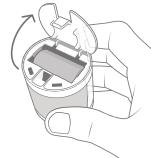
**EN** To replace the battery, simply open the battery compartment cover.
