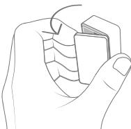
**EN** Simply remove the cover from the IntelliTAG™ and replace the battery.
